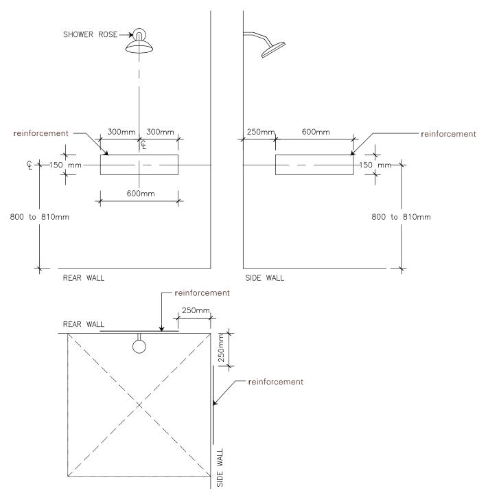
Figure 8(a) Shower recess - Location of reinforcement
