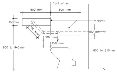
Figure 6(a) Toilet - Location of reinforcement
