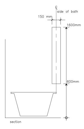
Figure 7(a) Bath – Location of reinforcement
