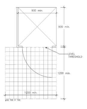
Figure 5(a) Gold level circulation space requirements for shower recess
